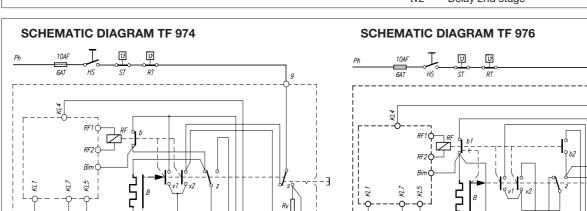
Ξ Rv Rv SA (₽ 54  $\bigcirc$ нŻ (0)ന hànd  $\sim$ V2 V1 HS Mains switch F Flame detector MZ 770 S OV Oil preheater ST Limit thermostat V Valves RF Flame relay RT Control thermostat Ζ Ignition B Thermomechanical timer SA Lock-out signal indicator M Burner motor **RV** Resistor
